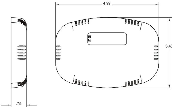
The H8800 from GRI is a single sensor programmable humidity monitoring security device. Unlike it's 1st cousin, the T8800, used for temperature sensing, the H8800 has one sensor to detect and report relative humidity. The single humidity sensor is housed in the appliance (H8800) or it can be ordered with a remote probe (H8800R). The memory in the H8800 is non-volatile.
